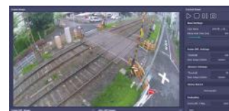
Railway crossing AI camera monitor
