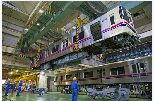
Maintenance of a Keio Line vehicle
