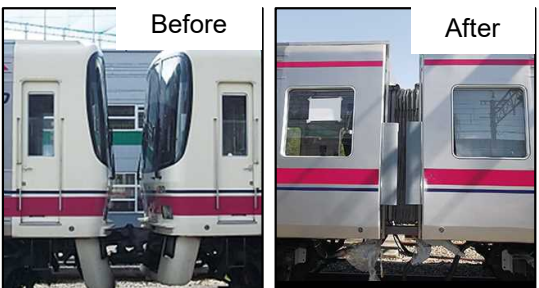
《Photo of railway car renovation to add connecting corridors》
