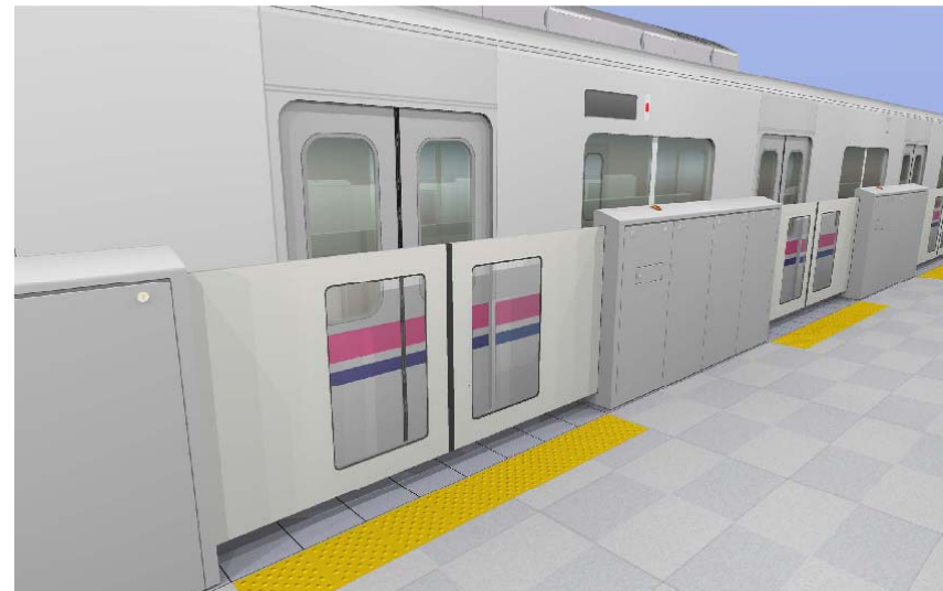
Platform doors installed in the Shinjuku Station (conceptual drawing)
