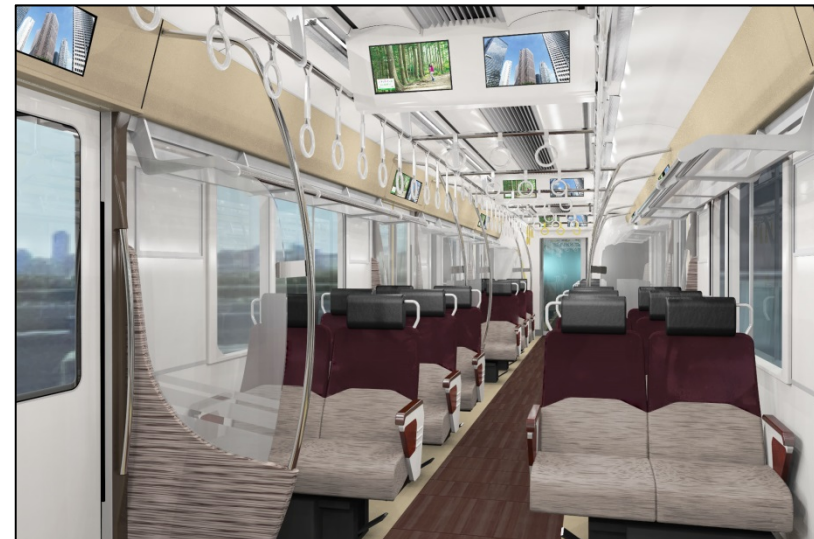
Seats can be converted from cross seats to long seats
